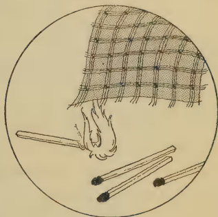
FIG. 204. — Wool burns slowly. This is a good way to test wool.
